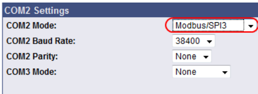
Figure 149: MODBUS – CS121 COM2 Settings
