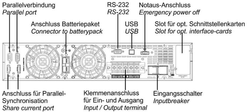
Figure 27: Rear view of XANTO 6000 and 10000
