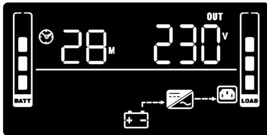
Figure 20: Battery mode display
