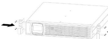
Figure 9: Securing the mounting bracket
